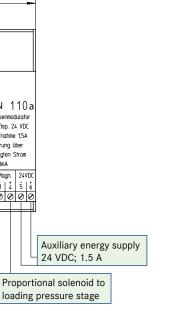
Outlet for the electric pilot 0/4 - 20 mA
