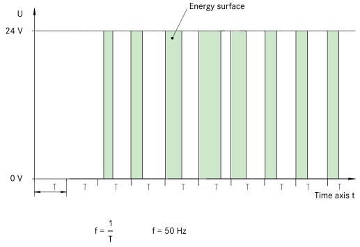
Actuation of the loading pressure stage
