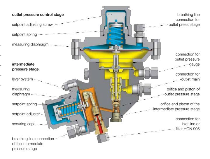
This two-stage regulator was designed to keep the outlet pressure of a gaseous medium constant in the main and independent of disturbing influences like inlet pressure or flowrate changes. Due to the intermediate pressure unit integrated into this spring-loaded regulator the negative influence of inlet pressure changes upon the regulating accuracy is reduced to a negligible minimum and practically excluded.
